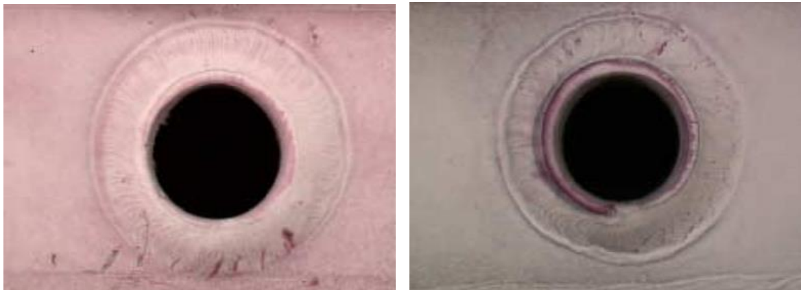
Figure 2 Dye penetrant results on the DSS 2205 tube to tubesheet welds
