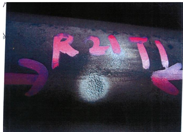
Figure 8 Several localised corrosion attack observed on Feed/BPA exchanger tube external as shown in the left picture and close up shown in the right picture.
