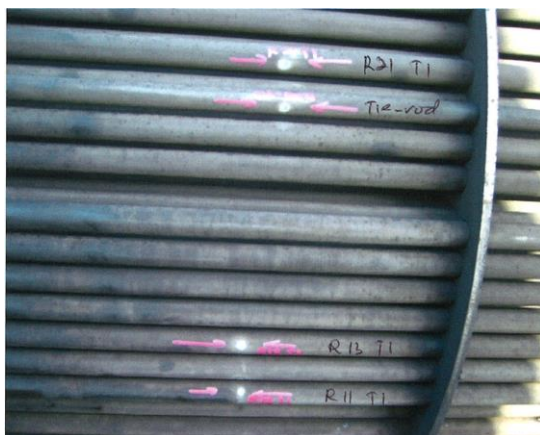
Figure 8 Several localised corrosion attack observed on Feed/BPA exchanger tube external as shown in the left picture and close up shown in the right picture.
